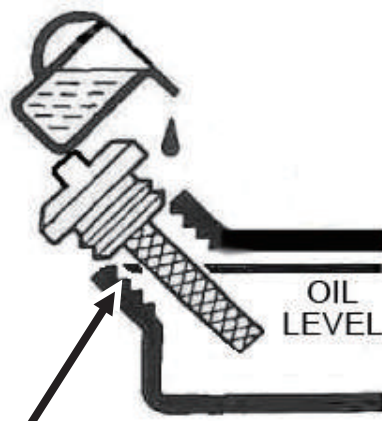
Figure 2 - Add Oil To TOP Of Threads
